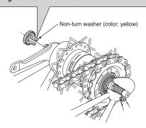
Screw the flange nuts onto both ends of the hub axle. After this, take up the slack in the chain and then tighten the flange nuts to secure the wheel to the frame.
