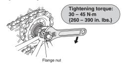
Check that the right end of the hub axle protrudes from the edge of the flange nut by about 8 - 12.5mm.
