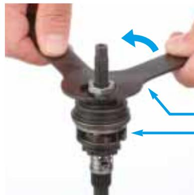
Remove the right hand lock nut and the right hand cone with dust seal from the hub axle.
