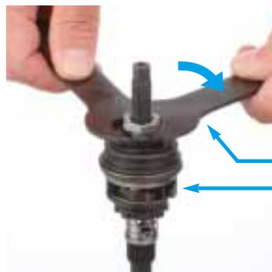
Install the right hand lock nut and the right hand cone with dust seal onto the hub axle.
