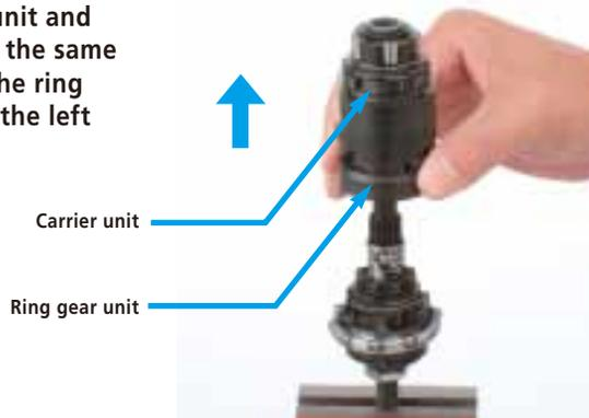
After removing them at the same time, remove the carrier unit from the ring gear unit.
